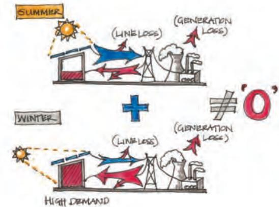
Figure 3. Source energy accounts for generation and transmission losses, but site energy does not.
