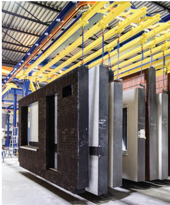
Panels in factory lined up and ready to be installed in an Energiesprong retrofit in the Netherlands.
