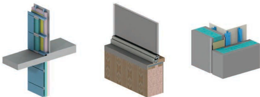
(left) Cantilevered balcony. (middle) Window sill transition. (right) Wall corner. (Courtesy of Morrison Hershfield Ltd)
